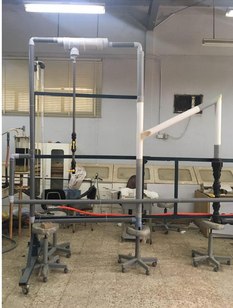
Figure 3-10 GLCC Test Section
