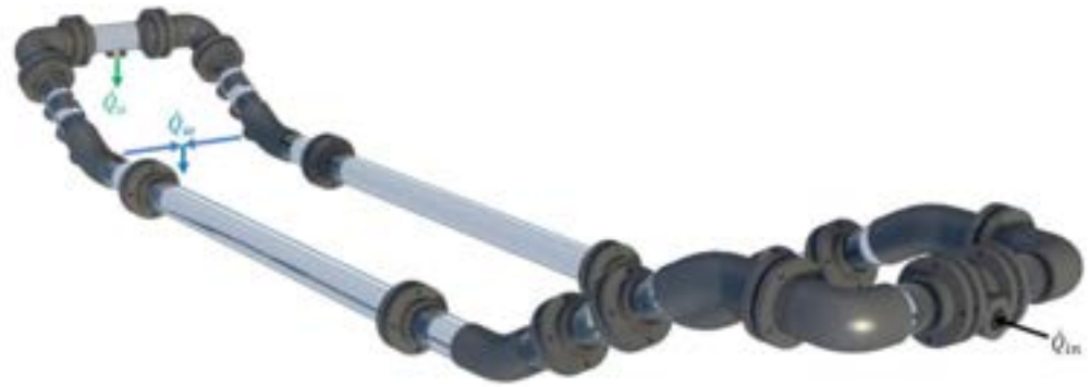
Figure 6. Prototype of parallel pipe bulk oil-water separator.
