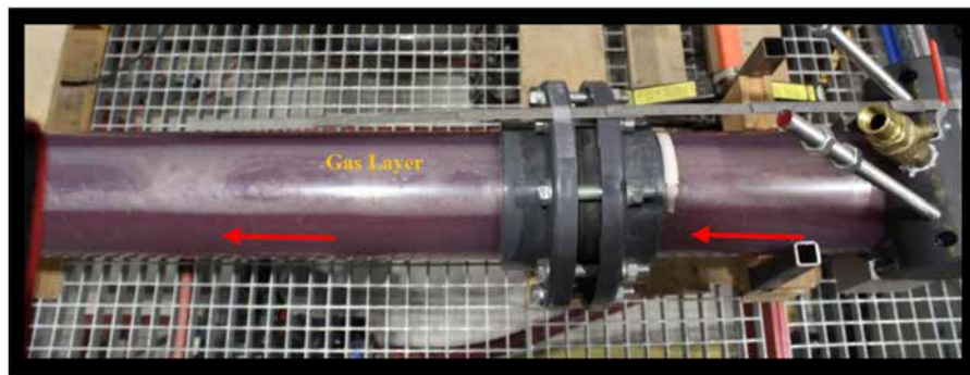
Figure 6—Decreasing the effective horizontal pipe cross section
